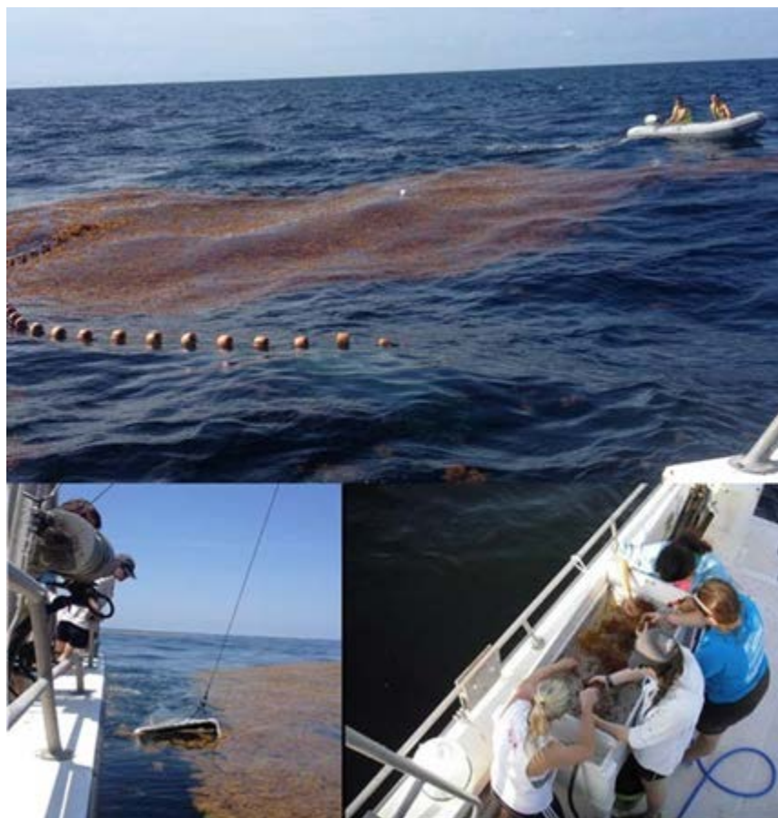
Figure 2. Plankton purse seine. Top: encircling Sargassum with a plankton purse seine; Bottom Left: collecting Sargassum with a neuston net; Bottom Right: Rinsing Sargassum in sorting trough.
