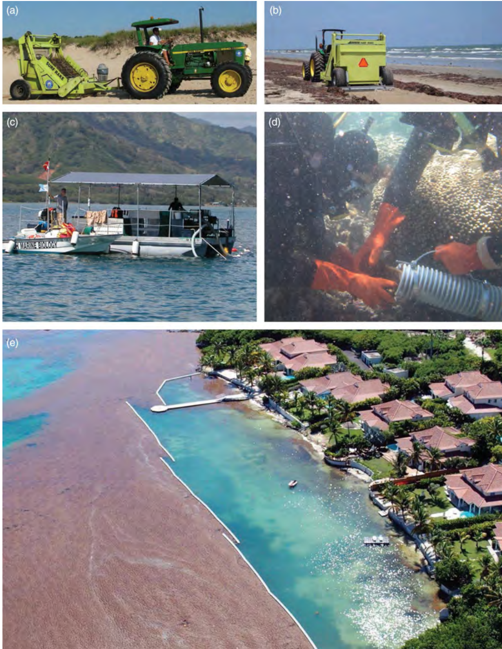
Figure 15.5 Some examples of mechanical methods for mitigating macroalgal blooms on beaches and in coastal waters. (a,b) The Barber surf rake used to remove macroalgae from beaches; Source: photos courtesy of H. Barber & Sons, Inc. (c,d) the “super sucker” used for removing invasive red macroalgae from coral reefs in Kane’ohe Bay, Hawai’i; Source: photos by B. Lapointe. (e) floating booms used to deflect pelagic Sargassum from coastal properties in the Caribbean. Source: photo courtesy of D. Jimenez.
