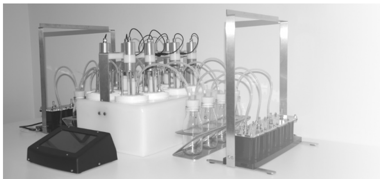
Figure 2. CJC biomethane potential system (courtesy CJC labs).
